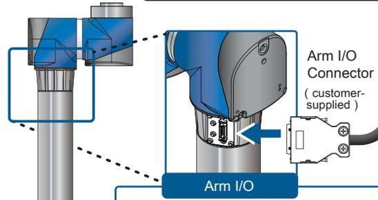
**!** Keep the current consumption of a device connecting to the Arm I/O to be no higher than 100 mA.
