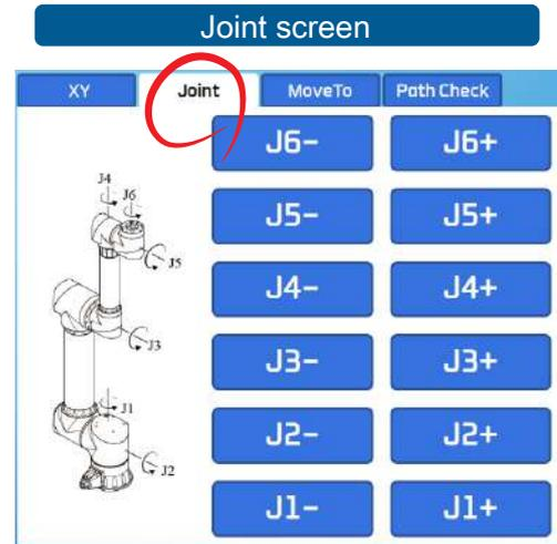
**Method 2** Operate to teaching point by **MoveTo Target** in joint coordinate system
