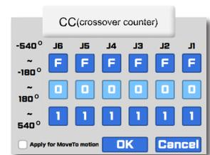
\*1) Crossover counter is the setting for covert posture data from cartesian coordinate system to joint coordinate system.
